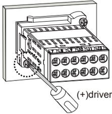
※Insert the unit into a panel, fasten the bolt with a (+) driver.
