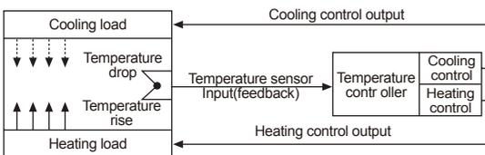
※For heating and cooling control, OUT1 control output is dedicated to heating control and OUT2 control output to cooling control.
