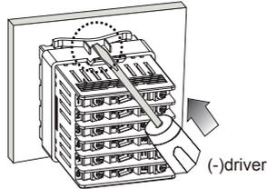
※Insert the unit into a panel, fasten the bracket by pushing with tools with a (-) driver.
