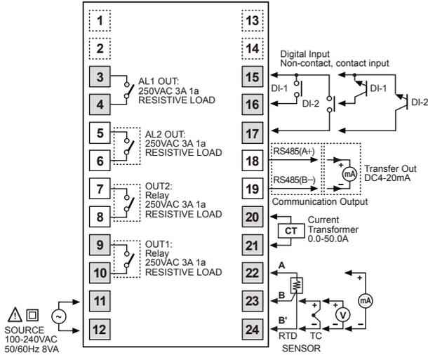
※Digital input is not electrically insulated from internal circuits, so it should be insulated when connecting other circuits. (Photocoupler, Relay, Independent switch)
