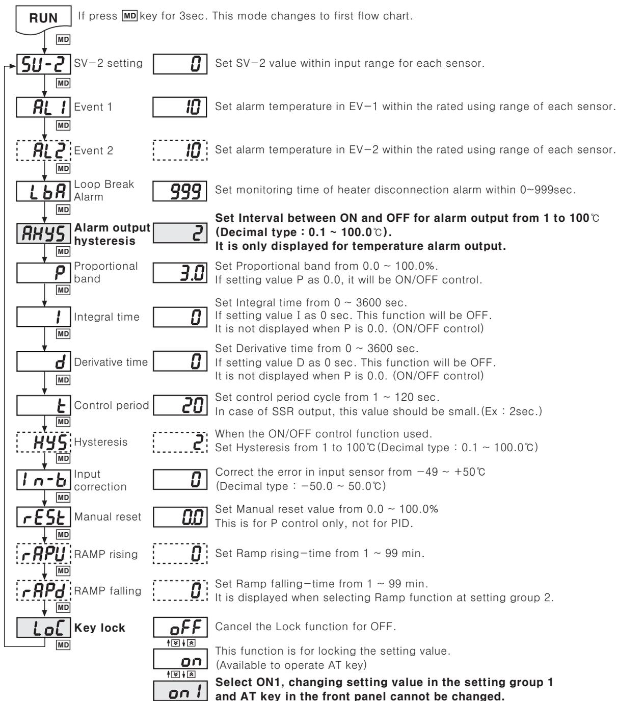
※ It will start to flash by pressing **◀** (◀) key and the flash will be moved by **◀** (◀◀), **▶** (▶▶) keys then set the value by **▲** (▲), **▼** (▼) keys. After that if pressing **MD** key the DATA will be changed then display next mode.
