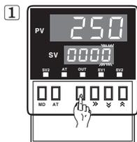
In case of changing the setting value at status of RUN, push ◀ (◀◀) key. 10<sup>0</sup> digit will flash at SV.
