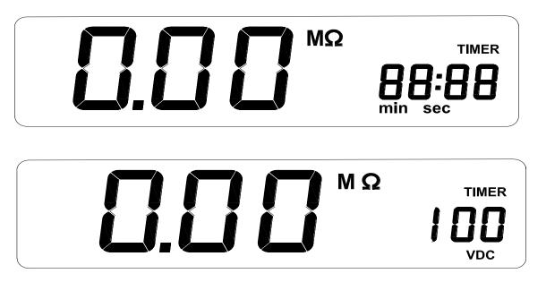
Press SELECT to check the preset time. The LCD screen display TIMER, PRES is shown on primary display, the secondary display shows the preset time. Press ENTER, the meter display Set. The time can be adjusted by  $\triangle/\nabla$  button. Presws ENTER again to confirm the adjustment.
