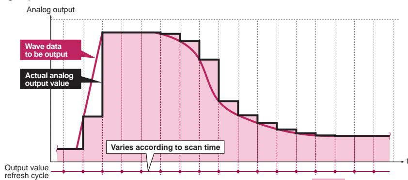
The actual analog output values are deviated from the target wave data.
